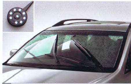
25 Rain sensor SEWAYA8000 E Activates wiper blades automatically.
