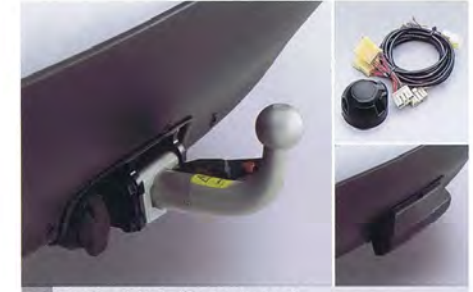
24 Trailer hitch (Detachable) See Application List W Maximum towing capacity 2,000 kg.
