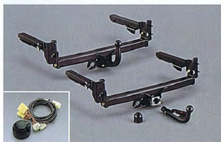
45 Trailer hitch (Fixed, Detachable) See application list W Maximum towing capacity 2,000 kg.
