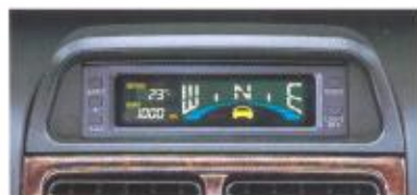
52 GAUGE PACK [with INSTRUMENT PANEL CASE] Displays compass, altitude, and outside temperature.
