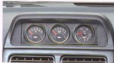
61 Sports gauge pack Oil thermo meter, oil pressure meter and boost meter
