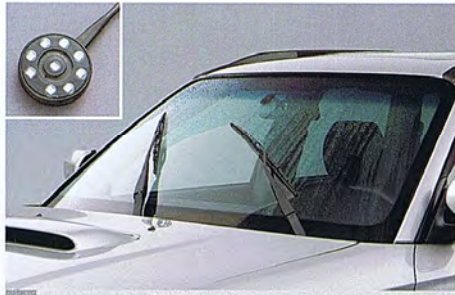
49 Rain sensor SEWAYA8000 E Activates wiper blades automatically.
