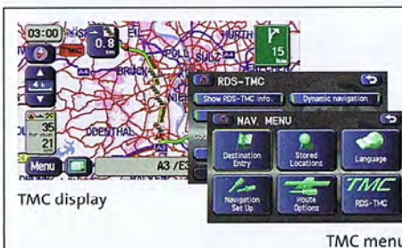
99 TMC unit (DVD Navigation) H001EAG102 W Provides traffic information and alternative routes avoiding traffic jams. *For DVD Navigation.
