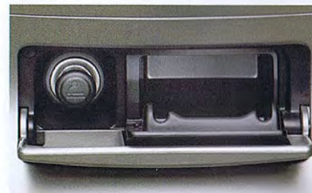
73 Smoker's kit H6010SA100 W Changes the accessory socket to a cigarette lighter, combined with an ashtray.
