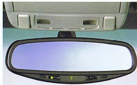
72 Auto-dimming compass mirror H501ESA000 W Includes electronic compass. Mirror darkens automatically when headlights are detected from the rear of the vehicle.
