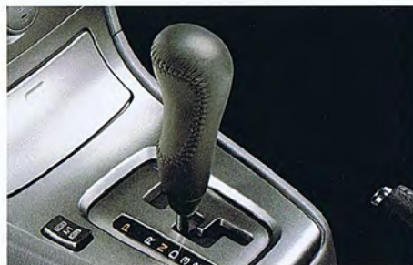
79 Leather shift knob (AT) 35126FE080 W Handsome leather-wrapped shift knob for automatic transmission.
