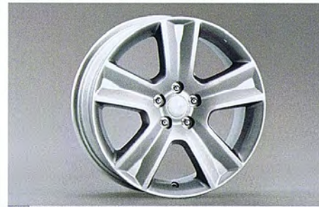
17 Alloy wheel 5-spoke (17 inch) 28111AG210 W 17x7JJ offset 48 215/55R17
