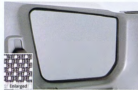
51 Rear sunshade (Side) F505ESA100 W Protects from sunshine and darkens your luggage compartment. Mesh type.
