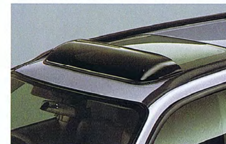
31 Sunroof deflector F541SSA000 W Helps reduce wind noise and cut sun glare.
