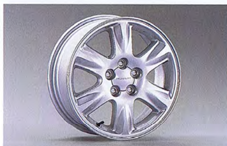
27 Alloy wheel 6-spoke (15 inch) 28111SA010 W 15x6JJ offset 48 205/70R15 – 195/70R15 (snow)
