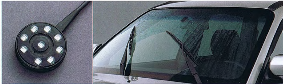
49 Rain sensor SEWAYA8000 E Activates wiper blades automatically.
