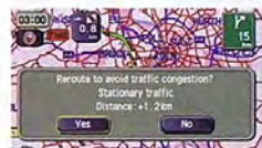
98 TMC unit (DVD Navigation) H001EAG102 W Provides traffic information and alternative routes avoiding traffic jams.
