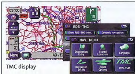
98 TMC unit (DVD Navigation) H001EAG102 W Provides traffic information and alternative routes avoiding traffic jams.
