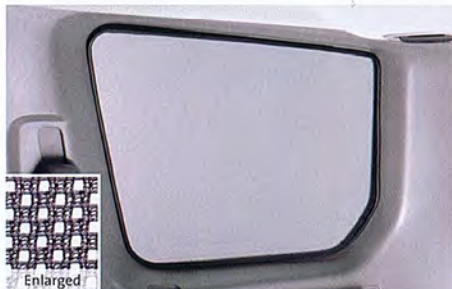
52 Rear sunshade (Side) F505ESA100 W Protects from sunshine and darkens your luggage compartment. Mesh type.
