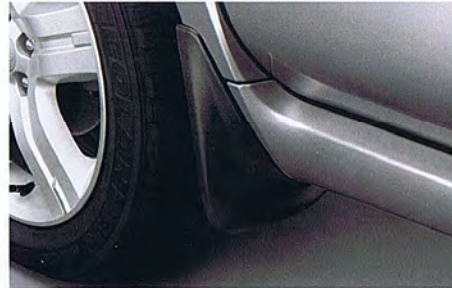
30 Splash guard (Front & Rear set) J101ESA300 W Helps protect your vehicle from mud and snow.
