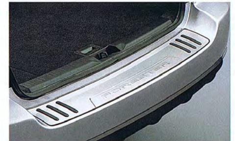
34 Cargo step panel (Stainless) E7710SA000 W Protects rear bumper from scratches.
