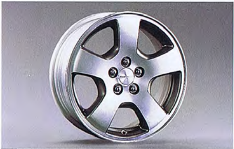
20 Alloy wheel 5-spoke (16 inch) 28111FC000 W 16x6.5JJ offset 48 215/60R16
